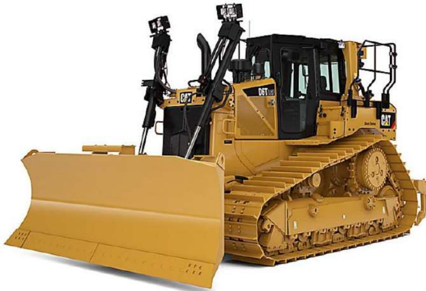
Figura 7. Tractor oruga (Bulldozer) 191/240 CV (CAT9)
